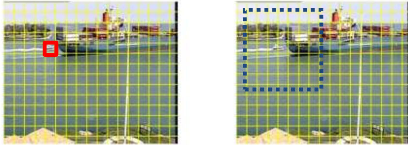
Figure 8 - Left: the current image with the block B_{p,q} highlighted. Right: the reference image. The search window centered in (p,q) is shown.
